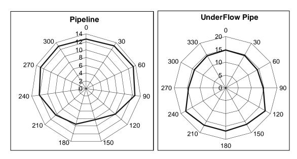
Figure 15: Pipe wall thickness in millimeters as a function of angular position from top of pipe as shown on two different pipes at a customer site
