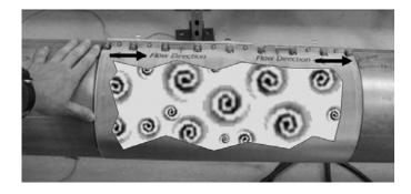
Figure 1: Cutaway of pipe under sonar array sensor band illustrating turbulent eddies
