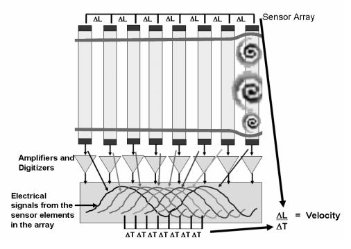
Figure 2: Illustration of signal detected by passive sensors in array from one collection of turbulent eddies.
