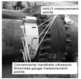
Figure 13: Pipewall thickness measurement points to compare conventional technique with  $HALO^{TM}$
