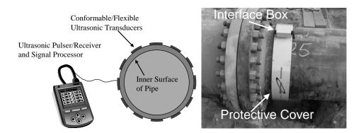
Figure 12: Conceptual layout of  $HALO^{TM}$  system and picture of system in operation at a customer site
