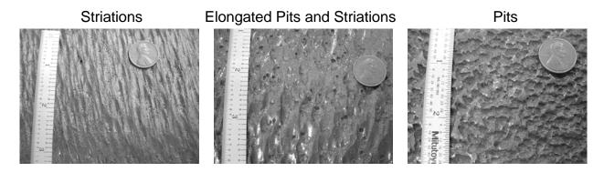
Figure 19: Inner surface irregularities seen on chromium-steel worn pipe
