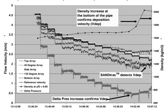
Figure 9: 186  $\mu m$  Slurry solid deposition detected by sonar meter, densitometer, and delta-pressure
