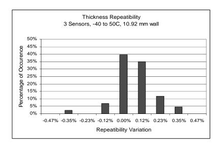
Figure 17: Small spread in data over 90C temperature range and over three sensors is shown
