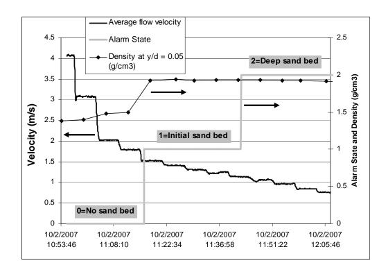
Figure 6: Alarm States – 89 µm slurry
