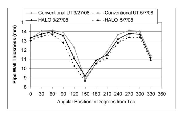
Figure 14: Conventional ultrasonic (UT) pipewall thickness measurement versus  $HALO^{TM}$  measurements
