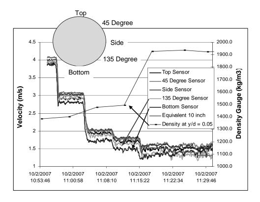
Figure 5: Velocity profile of 89 μm mining slurry.
