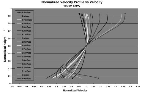
Figure 11: Velocity profiles (normalized to pipe center velocity) vs. reference velocity
