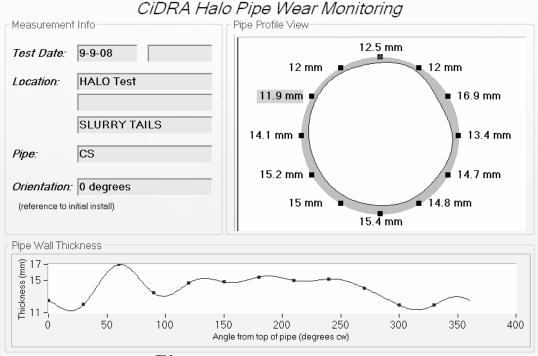
Figure 16: HALO<sup>TM</sup> pipe wall thickness visualization software output
