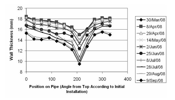
Figure 18: Measurement of pipe wall thickness as a function of angular position and time is shown
