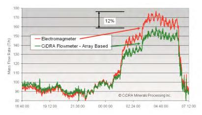
Figure 7. Impact of ferromagnetic slurry on mass flow rate, showing over-reporting by electromagnetic based flowmeter versus array based flowmeter
