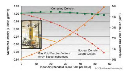
Figure 12. Nuclear density gauge correction using array-based meter
