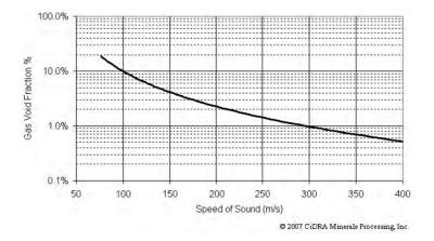
Figure 5. Example of relationship between gas void fraction (entrained air bubbles) and speed of sound
