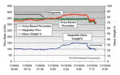
Figure 6. Electromagnetic flowmeter erroneously respond to magnetite whereas array flowmeter accurately reports flow
