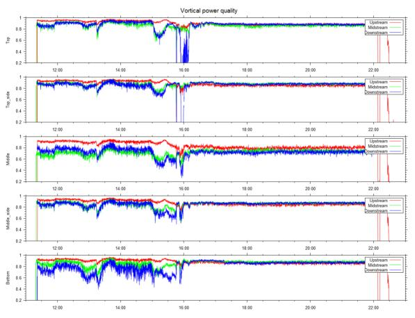
Figure 5 Vortical power quality data in turbulent and laminar flow of thick tailings.
