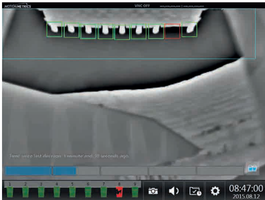
Using thermal imaging, MotionMetrics' LoaderMetrics detects a missing bucket tooth
