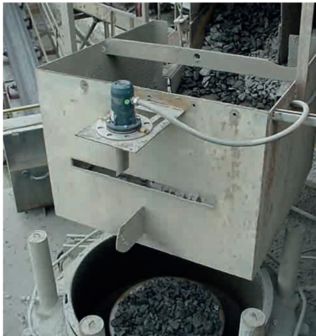
The ABB LM80 laser level transmitter is specifically designed for heavy industrial applications, such as here in a rock crusher level control application
