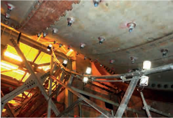
Impactmeter acoustic sensors installed on a SAG mill
