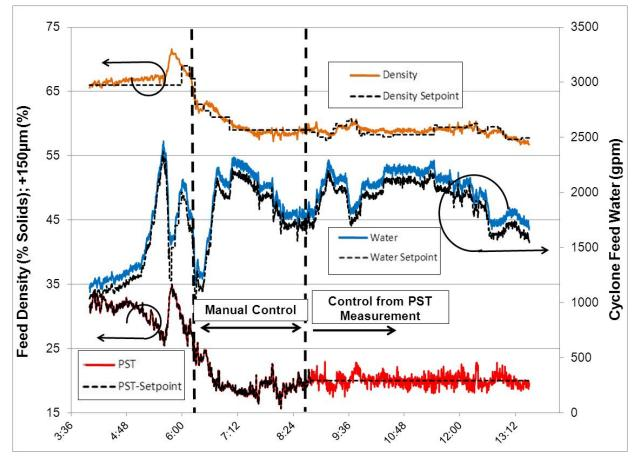
Figure 8 Manipulating density for PST control
