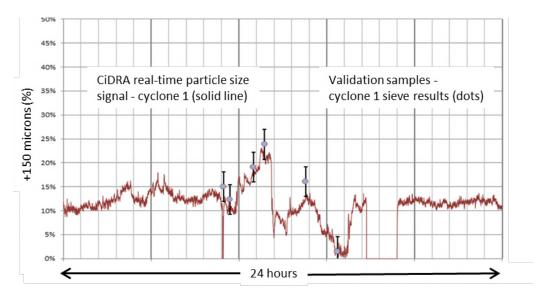
Figure 13 Hydrocyclone 1 CiDRA CYCLONEtrac PST signal vs. validation sieve samples
