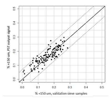
Figure 14 Percent Mass Fraction +150 micron, CYCLONEtrac PST output vs. validation sieve samples
