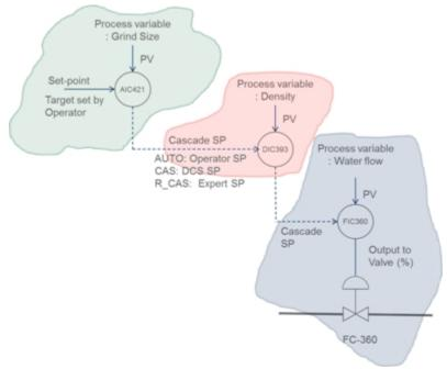
Figure 7 Cascaded control loops used to optimize grind value
