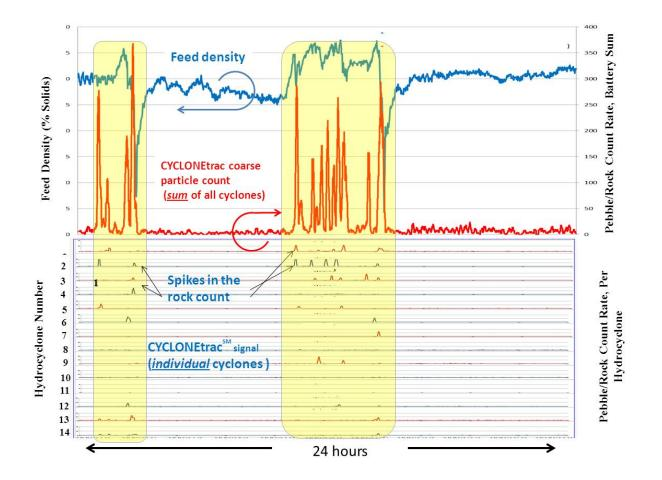
Figure 3 Multiple hydrocyclones cause the combined overflow of the battery to display spikes in the pebble/rock trend, which is coincident with increases in feed density to the battery.
