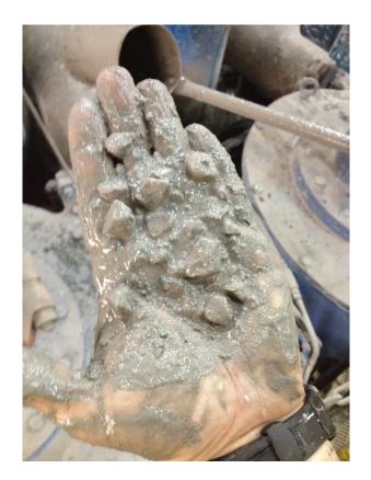
**Figure 6** During field validation, 78 samples were analyzed and compared to CYCLONEtrac OSM pebble counts. Shown is an example of material collected during a pebbles/rocks event.
