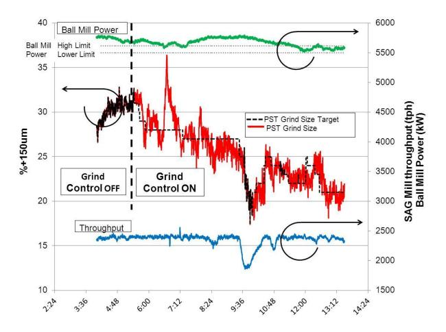
Figure 9 Reduction of grind size with constant TPH and target ball mill power
