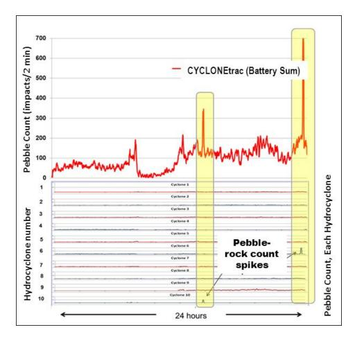
Figure 2 Single hydrocyclone causes combined overflow of the battery to display a spike in the pebble/rock trend.
