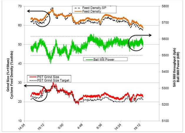
Figure 10 Example of particle size tracking leading to density setpoint changes and then to ball mill power draw
