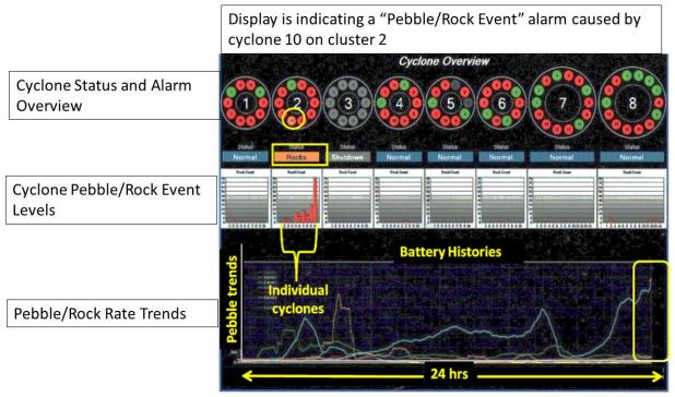
Figure 1 CYCLONEtrac OSM display with battery and individual hydrocyclone pebble/rock status
