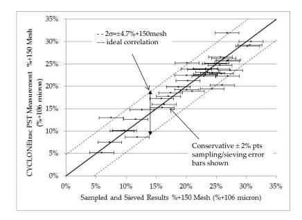
Figure 5 CYCLONEtrac PST 106 micron measurements compared to the sieved samples for a gold concentrator
