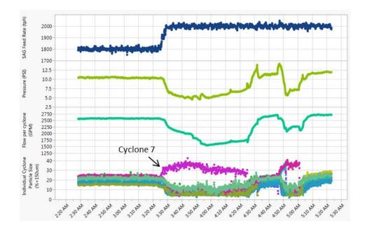
Figure 3 Example of a poorly performing cyclone
