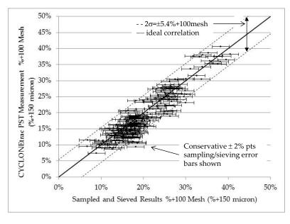
Figure 4 CYCLONEtrac PST 150 micron measurements compared to the sieved samples for a large copper concentrator
