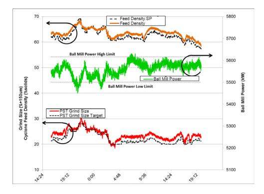
Figure 2 Example of CYCLONEtrac PST based control
