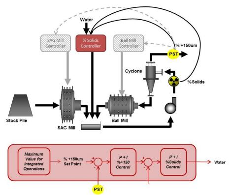
Figure 11. Example of battery level particle size control using CYCLONETRAC PST measurement.
