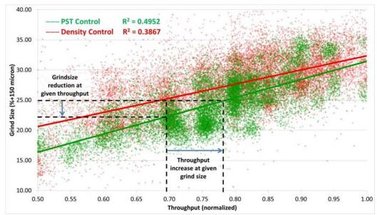
*Figure 12. Impact of using control enabled by CYCLONEtrac PST measurement compared with traditional density control.*
