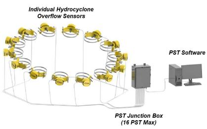
*Figure 2. Illustration of particle sizing system.*
