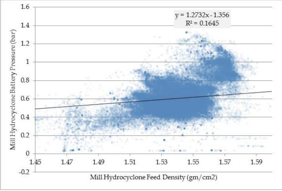
*Figure 10. Cyclone pressure plotted versus cyclone feed density.*
