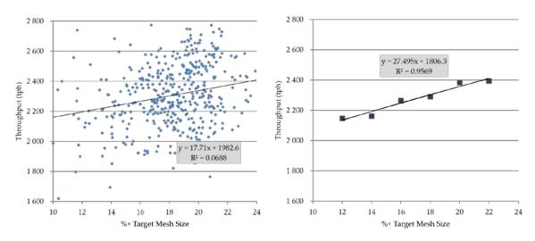
Figure 6 Throughput vs Product Size, with and without data binning
