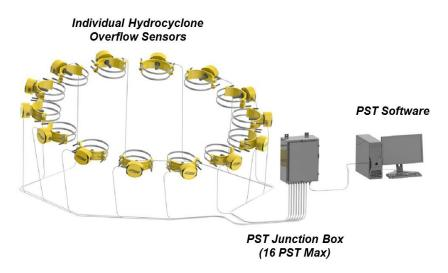
Figure 2 PST plant scale installation diagram
