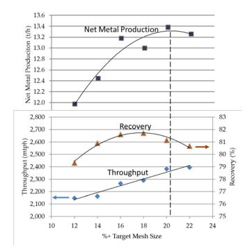
Figure 8 Net Metal Production (NMP) objective function (top) per Equation 1
