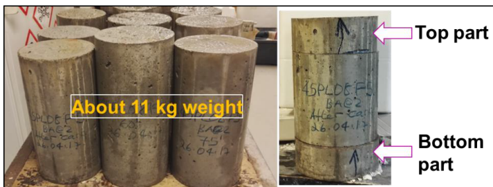
Figure 24. Example of the specimens used for sensitivity of concrete for segregation test.
