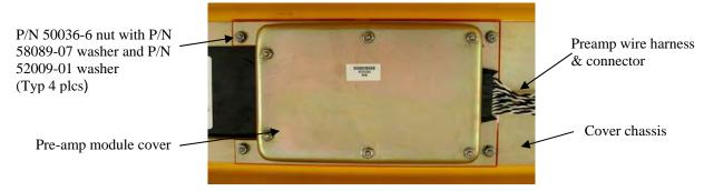
Figure 1 Pre-amplifier Module Installed In Sensor Cover
