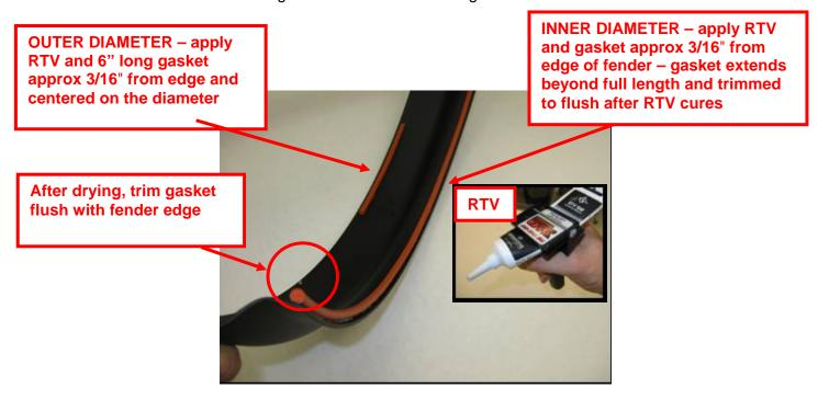
Figure 1 Fender Rework
