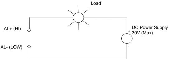
Figure 2 Example Alarm Circuit Diagram With Load 100mA Maximum
