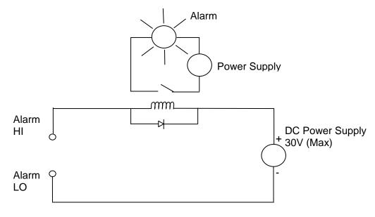
Figure 3 Example Alarm Circuit Diagram With Load Greater Than 100mA
