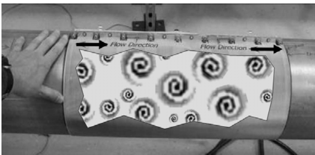
Figure 1. Cutaway of pipe under sonar array sensor band illustrating turbulent eddies
