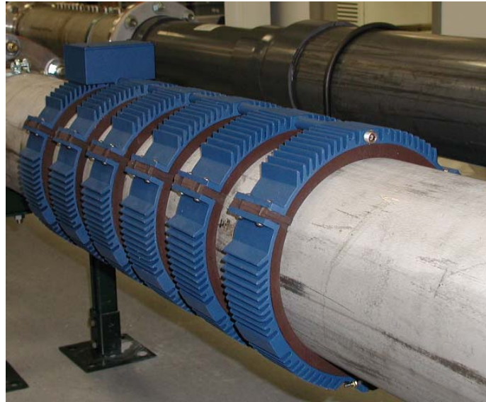
Figure 6: Photograph of an 8-inch diameter Sonar-based flow meter using six Clamp-on strain-based sensors
