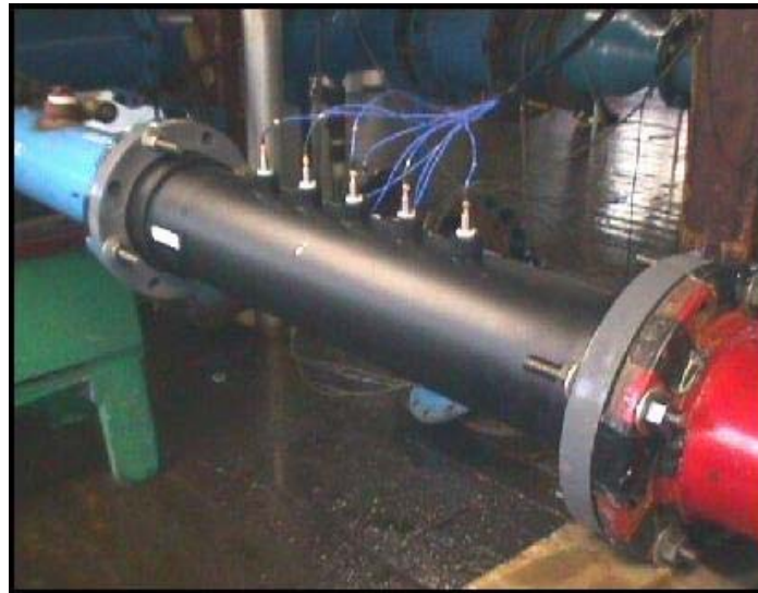
Figure 3: Photograph of a 6-inch diameter Sonar-based flow meter using 5 ported pressure transducers
