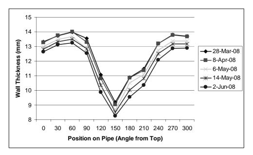
Figure 13: Measurement of pipe wall thickness as a function of angular position and time is shown
