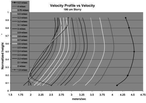
Fig. 8: Velocity profiles vs reference velocity
