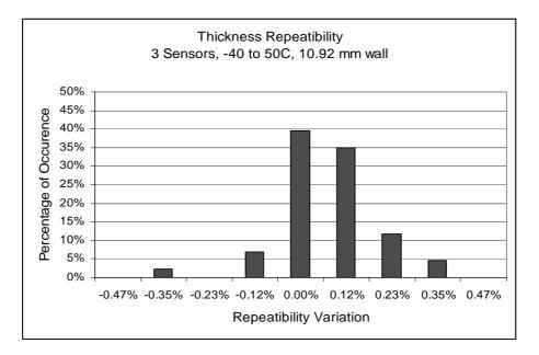
Figure 12: Small spread in data over 90C temperature range and over three sensors is shown
