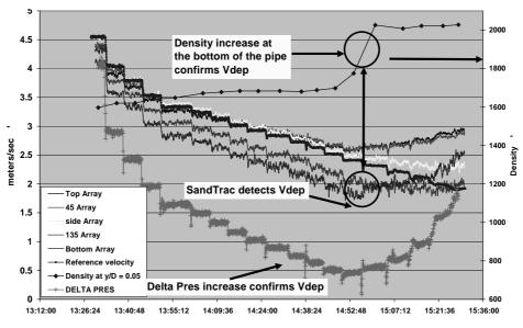
Fig. 7: Solid deposition detected by sonar meter, densitometer, delta-pressure
