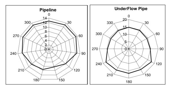
Figure 11: Pipe wall thickness as a function of angular position from top of pipe as shown on two different pipes at a customer site
