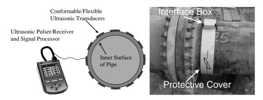
Figure 10: Conceptual layout of  $HALO^{TM}$  system and picture of system in operation at a customer site
