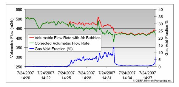
Figure 11 - Detection of entrained air bubbles and compensation of flow measurement
