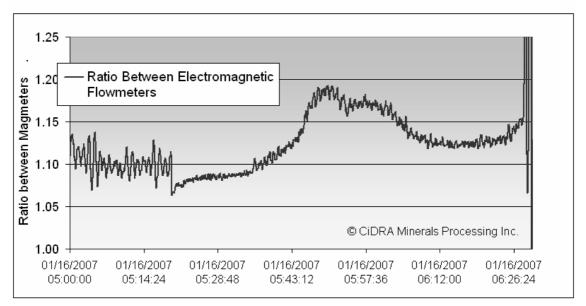
Figure 8 - Two electromagnetic flowmeters in series with array-based flowmeter showing offsets ranging from 2% to 18% between two electromagnetic flowmeters and accurate measurement provided by array-based flowmeter
