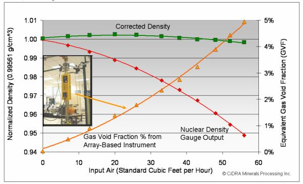
Figure 12 - Nuclear density gauge correction using array-based meter
