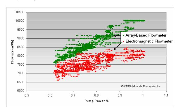
Figure 10 – Flow rate reported by array-based flowmeter and electromagnetic flowmeter relative to pump power (as percentage of maximum power)
