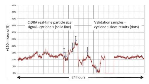
Figure 7 Hydrocyclone 1 CiDRA CYCLONEtrac PST signal vs. validation sieve samples
