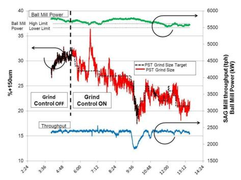
Figure 3 Reduction of grind size with constant TPH and target ball mill power
