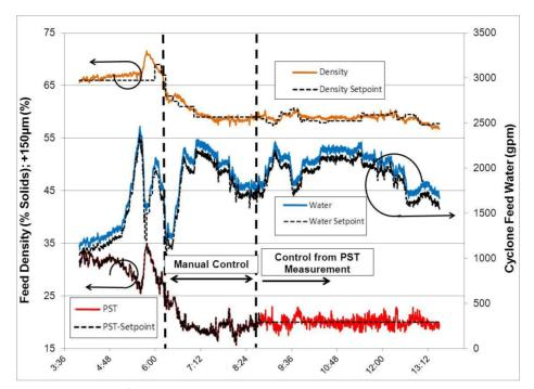
Figure 2 Manipulating density for PST control
