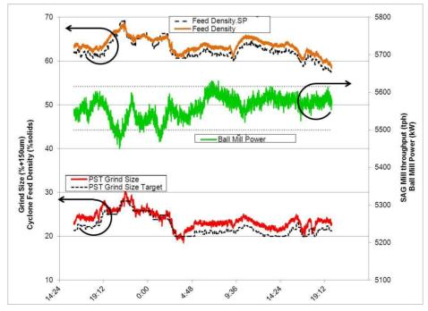
**Figure 4** Example of particle size tracking leading to density setpoint changes and then to ball mill power draw
