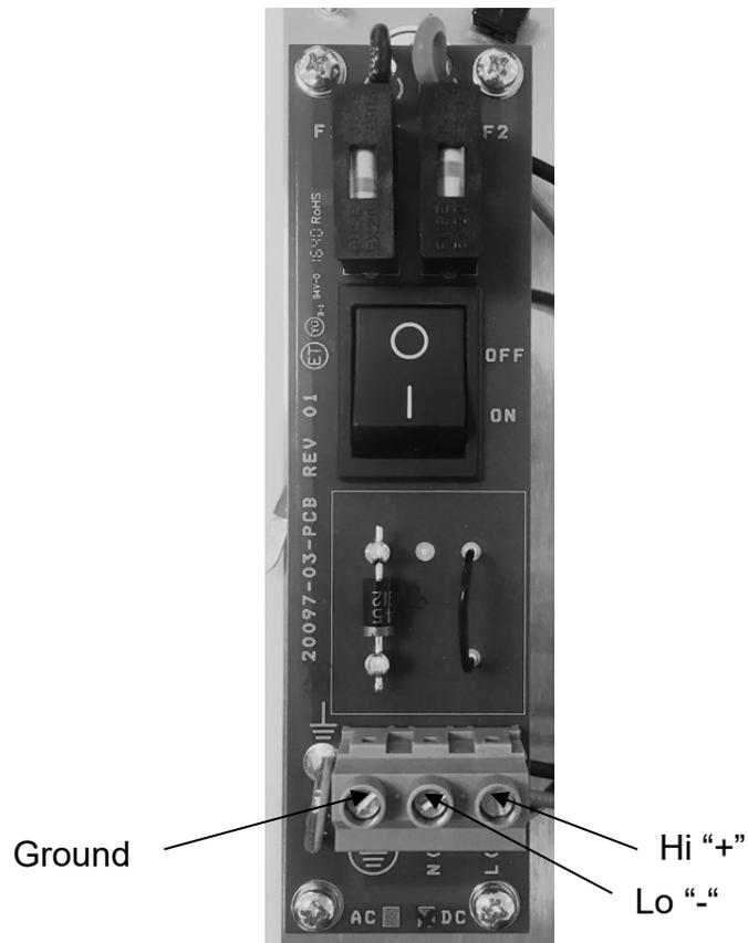
**Figure 18: Junction Box DC Power connection**
