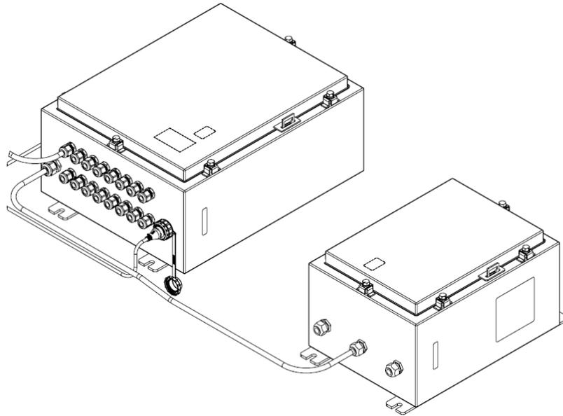
**Figure 15: 24VDC Power to Junction Box**
