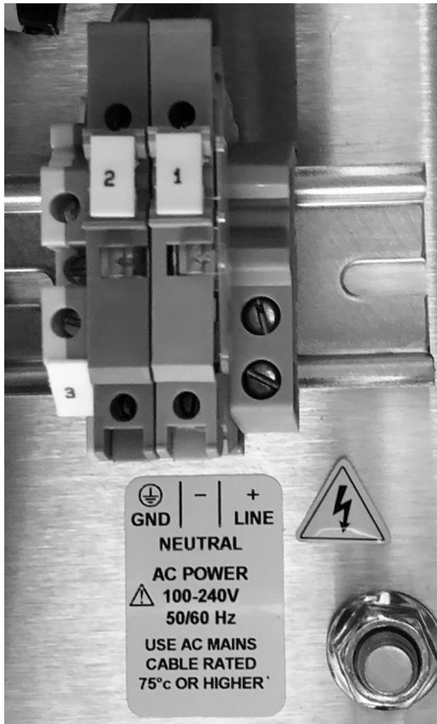
**Figure 14: Mains Power Connection**
