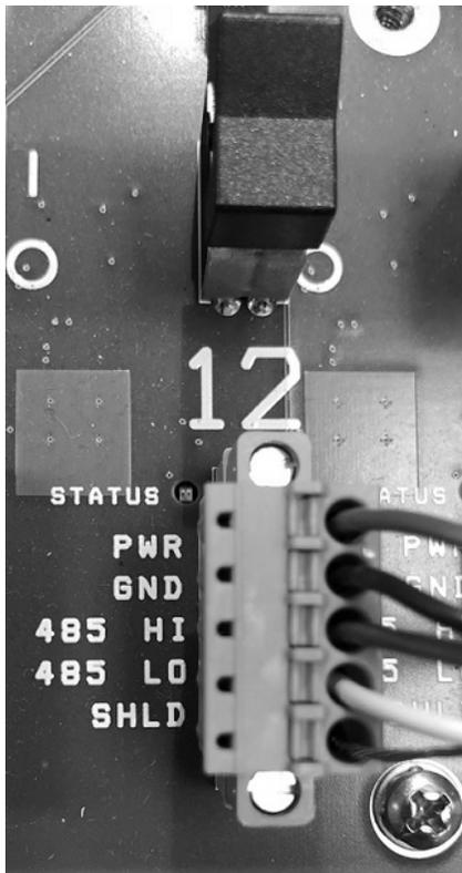
**Figure 23: Sensor Cable Connection to Junction Box Terminals**
