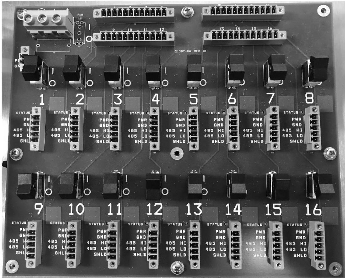
Figure 22: Terminal Block Numbering 1-8, 9-16
