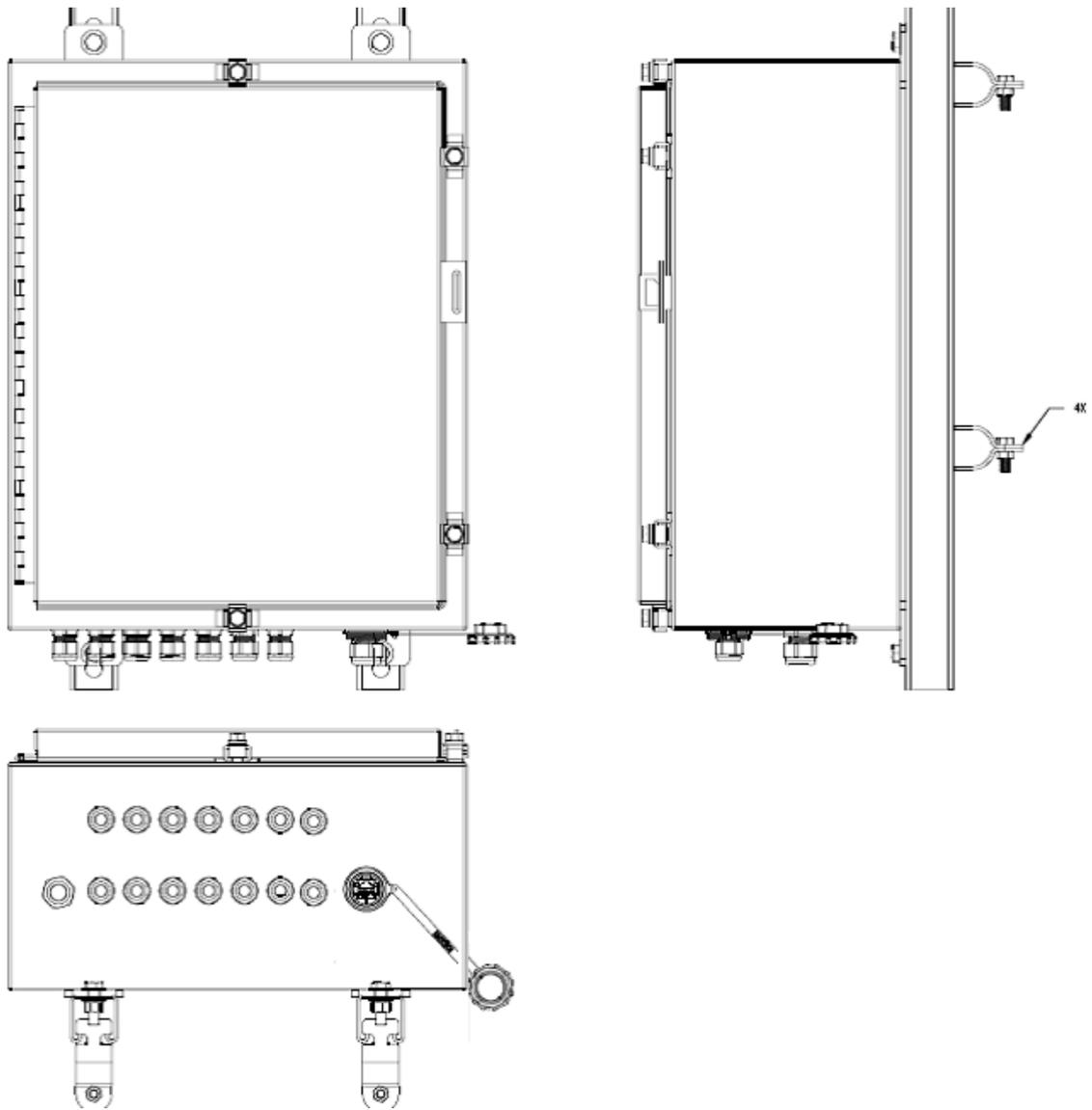
**Figure 5: Junction Box Mounting**
