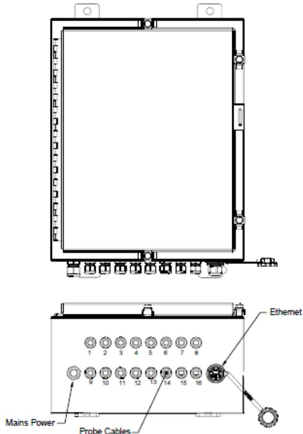
**Figure 11: Junction Box Connections**
