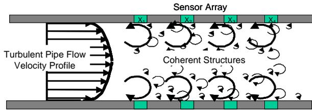
**Figure 1: Coherent Structures within Turbulent Pipe Flows**
