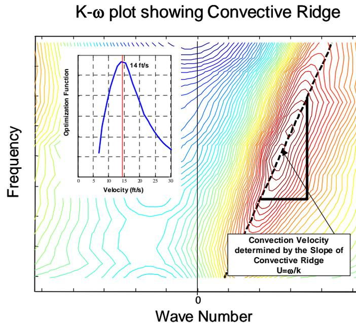
**Figure 2: K- $\omega$  plot generated from an array of sensors listening to water flowing in a 6 inch pipe at ~1000gpm.**
