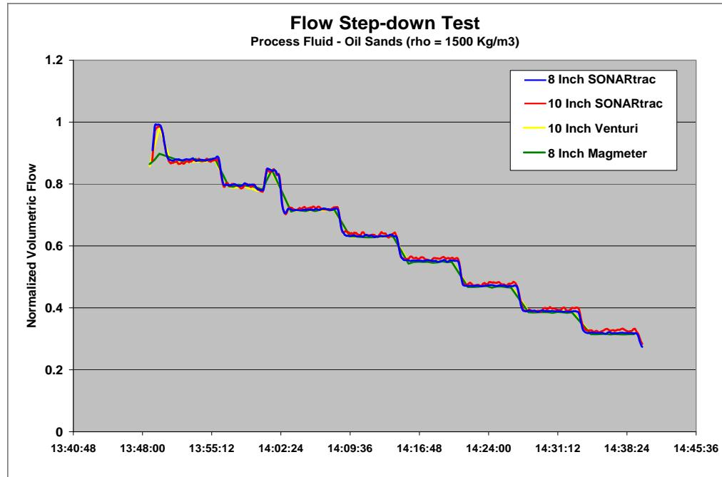
Figure 6: Flow Step-Down Tests
