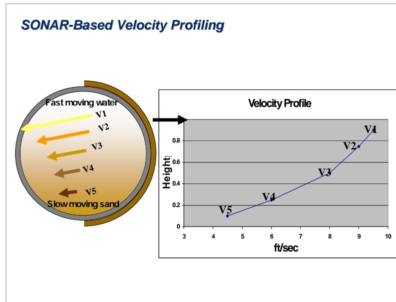
**Figure 15 SONAR-Based Velocity Profile**
