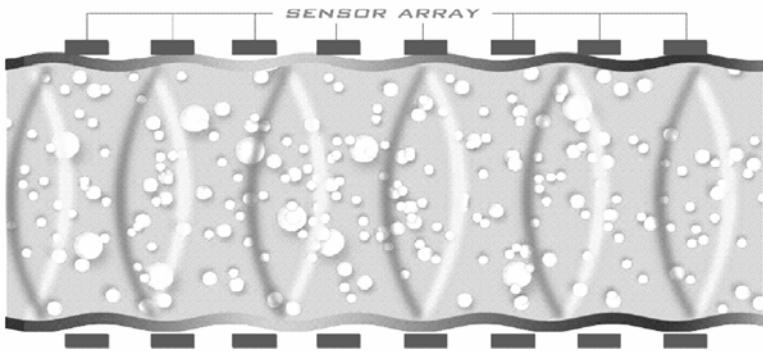
**Figure 3: Illustration of Naturally Occurring Acoustic Waves Propagating in Pipe under the Sonar Array Sensors**
