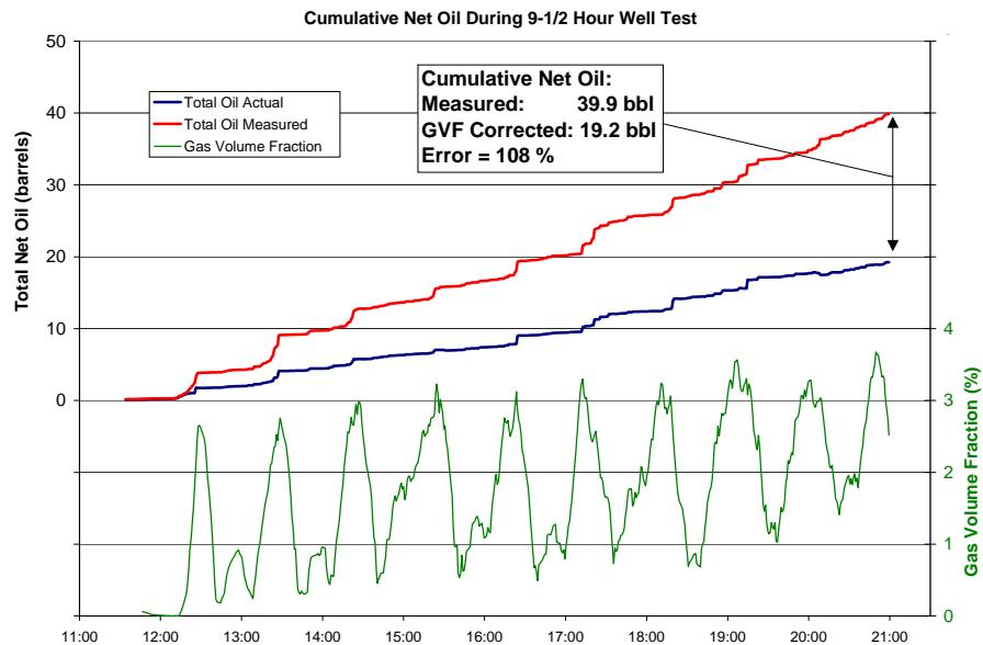
**Figure 12: Cumulative Net Oil, Reported and Corrected, and Gas Volume Fraction During Well Test**
