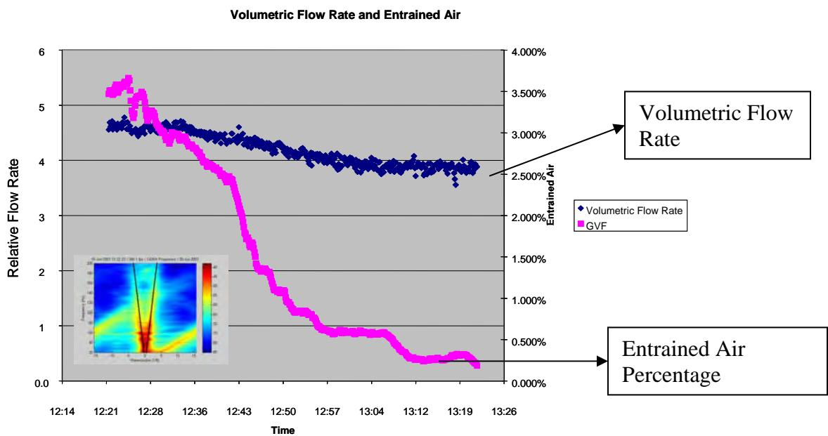
**Figure 7: SONARtrac Technology: Dual Measurements of Flow and Entrained Air Percentage (Gas Volume Fraction or GVF)**
