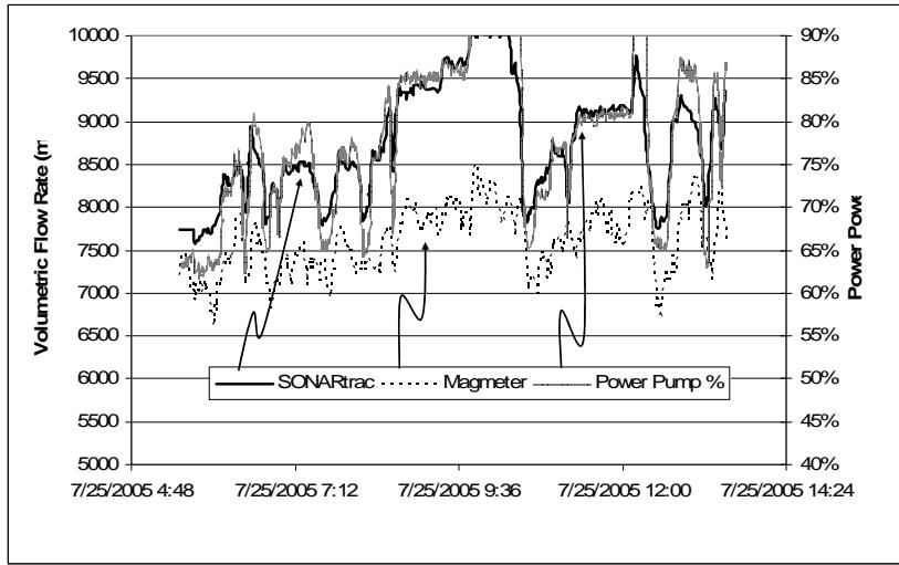
**Figure 13: Comparison of Sonar- Based Flowmeter with Magmeter and Pump Power Showing Excellent Correlation between Sonar- Based Flowmeter and Pump Power**
