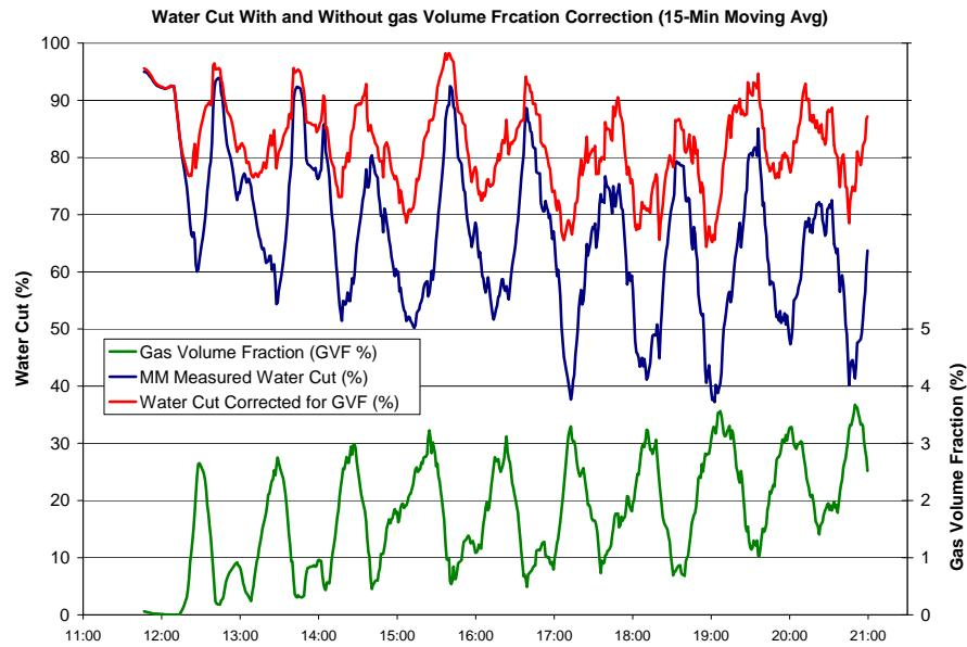
**Figure 11: Reported and Corrected Coriolis Watercut and Gas Volume Fraction During Well Test**
