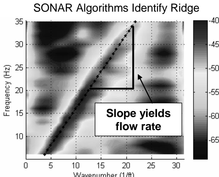
**Figure 2: Representative  $k$ - $\omega$  Plot Showing Convective Ridge**
