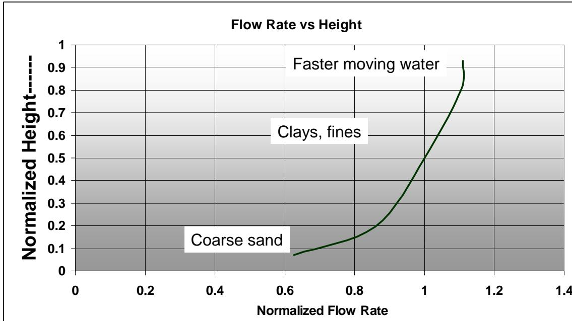
**Figure 16 Oil Sands Slurry Velocity Profile**
