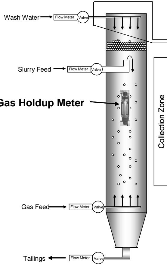
**Figure 17 (Left) Picture of Gas Holdup Meter and (Right) Diagram of Column Cell with Typical Location for Gas Holdup Meter**
