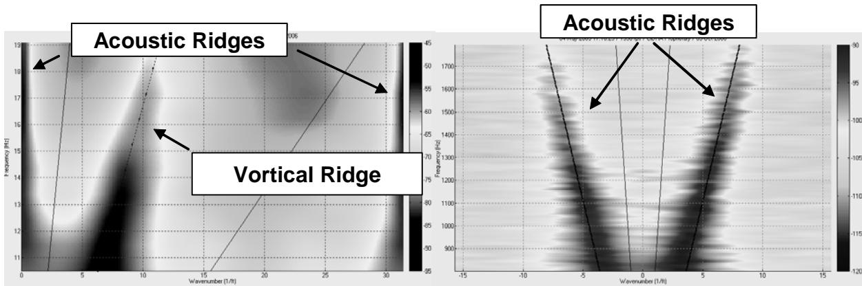
**Figure 4: (Left)  $K\omega$  Plot Showing Both Acoustic Ridges and Vortical Ridge (Right) Rescaling of Graph and Change in Frequency Range Enhances View of Acoustic Ridges**
