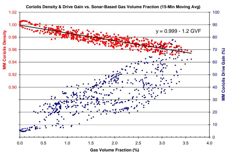
**Figure 10: Coriolis Density and Drive Gain Plotted vs. SONAR-based Gas Volume Fraction During Well Test**
