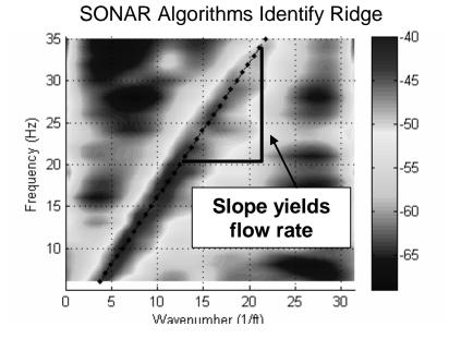
Figure 2: Representative k- $\omega$  Plot Showing Convective Ridge
