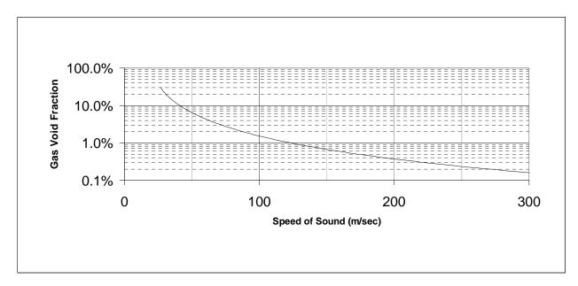
Figure 5: Example of Relationship between Gas Void Fraction and Speed of Sound
