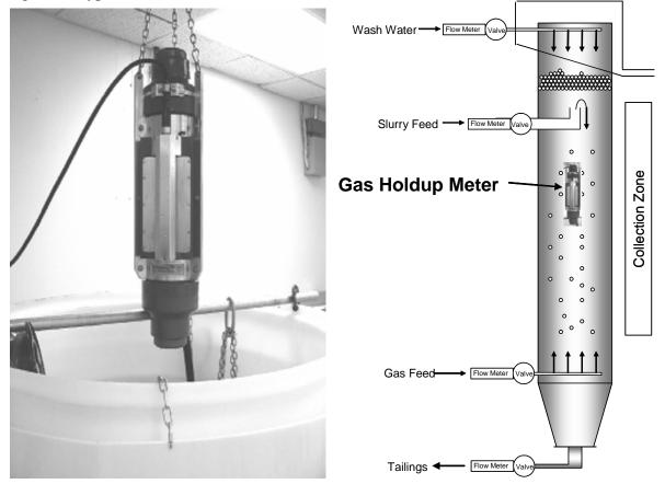
Figure 17 (Left) Picture of Gas Holdup Meter and (Right) Diagram of Column Cell with Typical Location for Gas Holdup Meter
