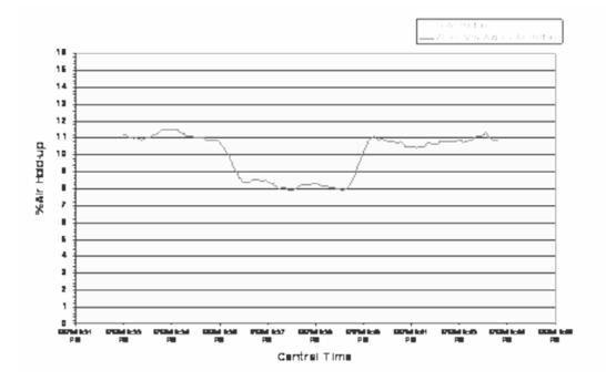
Figure 18 Gas Holdup "Bump" Test in Copper Flotation Column (Y-Axis Range is 0% to 18% Gas Holdup)
