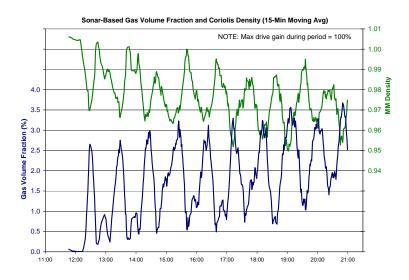
Figure 9: Coriolis Density and SONAR-based Gas Volume Fraction Reported During Well Test
