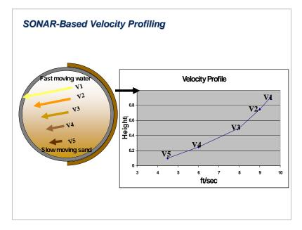
Figure 15 SONAR-Based Velocity Profile
