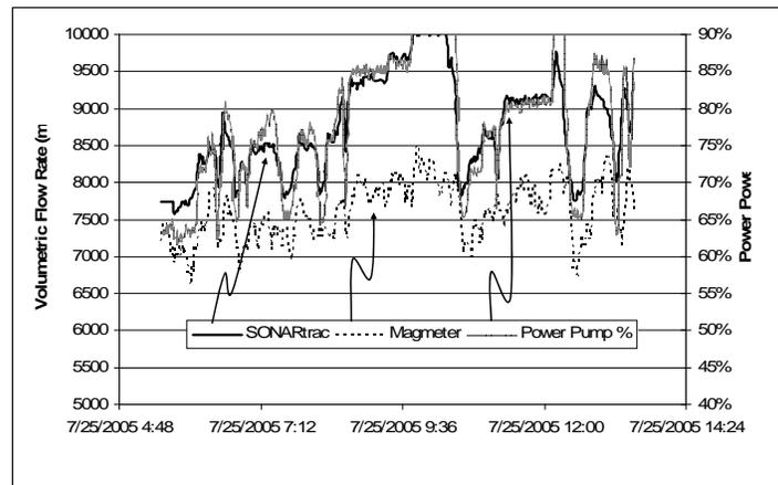
**Figure 5 Comparison of Sonar- Based Flowmeter with Magmeter and Pump Power Showing Excellent Correlation between Sonar- Based Flowmeter and Pump Power**
