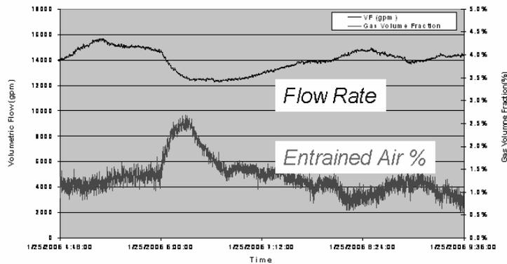
**Figure 93 Hydrocyclone Feedline - Accurate Flow Rate and Entrained Air Measurement**
