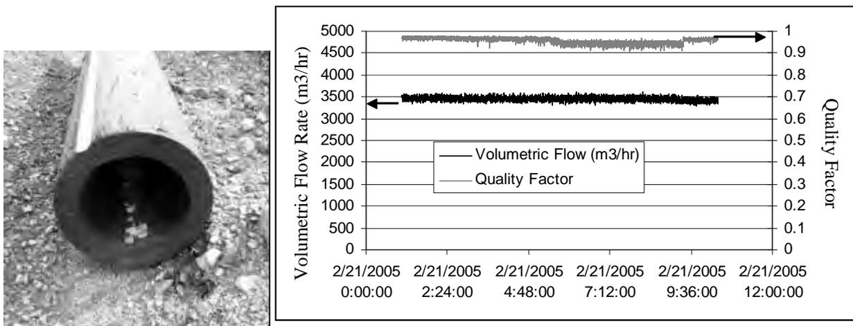
**Figure 7 Flow Measurements of Raffinate in a 30 inch High Density Polyethylene Pipe. Wall Thickness is 22.25 inches (5.6cm)**
