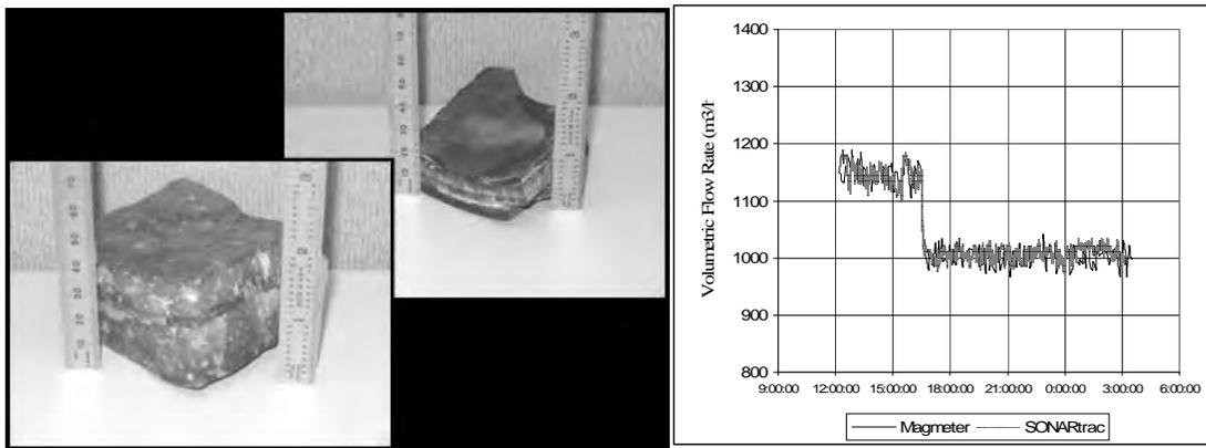
**Figure 6 Examples of Scale Buildup and Sonar- Based Flowmeter Operation in Water Pipe with Five Centimeters of Scale Buildup. Comparison to Recently Cleaned Magmeter is Shown.**
