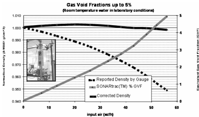
**Figure 14 Correction of Nuclear Density Gauge by SONARtrac™ Gas Void Fraction Measurement**
