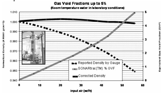
Figure 6 Nuclear density gauge correction using sonar-array based meter
