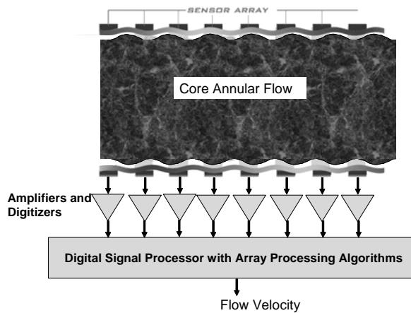
Figure 2 Diagram of pipe showing core annular flow with density variations and waves at core to annular interface
