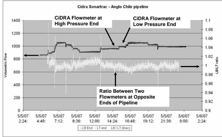
Figure 5 Results of leak detection using sonar array-based flowmeters in which overlapping dark lines are flowmeter outputs and the light line is the ratio between the two outputs.
