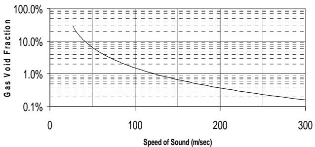
Figure 4 Example of relationship between gas void fraction (entrained air content) and speed of sound
