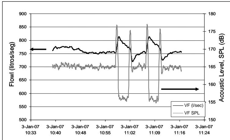
Figure 8 Flow Measurement and Acoustic Level Measurement for Valve Movement Monitoring at Choke Station
