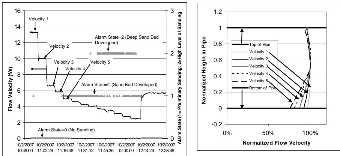
Figure 9 (Left) Normalized velocity profiles at various flow rates showing a drop in velocity at the bottom of the pipe at the lower flow rates. (Right) Flow velocity & alarm condition for low levels of sanding (Alarm level=1) and high levels of sanding (Alarm level=2)
