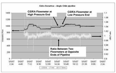
Figure 5 Results of leak detection using sonar array-based flowmeters in which overlapping dark lines are flowmeter outputs and the light line is the ratio between the two outputs.
