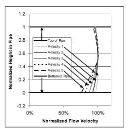
Figure 9 (Left) Normalized velocity profiles at various flow rates showing a drop in velocity at the bottom of the pipe at the lower flow rates. (Right) Flow velocity & alarm condition for low levels of sanding (Alarm level=1) and high levels of sanding (Alarm level-2)
