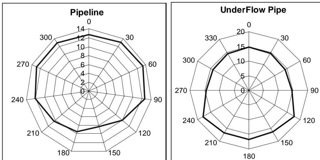
Figure 11: Pipe wall thickness as a function of angular position from top of pipe as shown on two different pipes at a customer site
