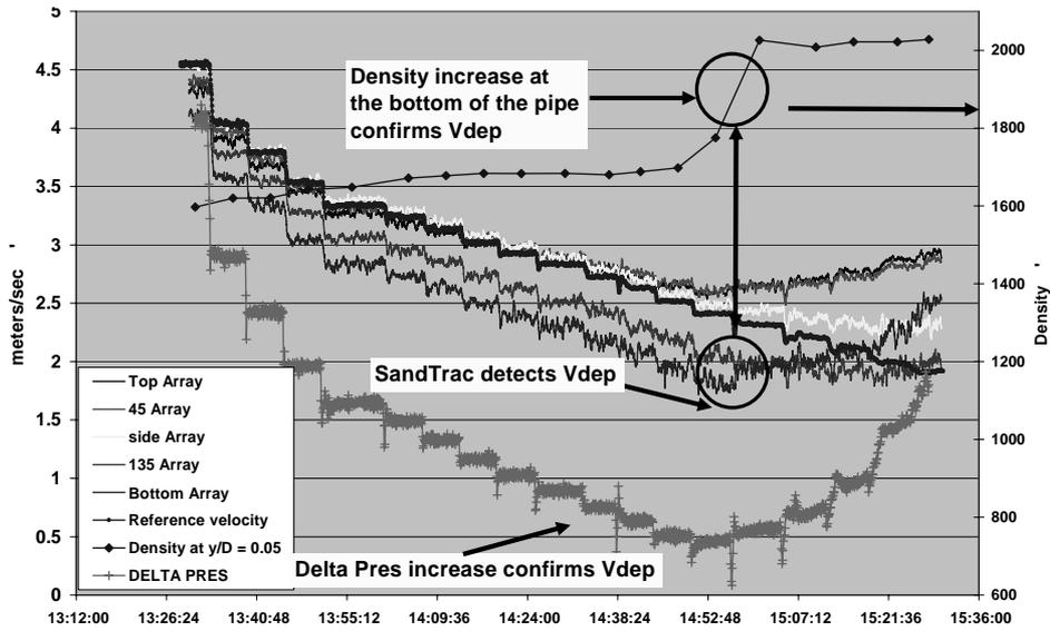
Fig. 7: Solid deposition detected by sonar meter, densitometer, delta-pressure
