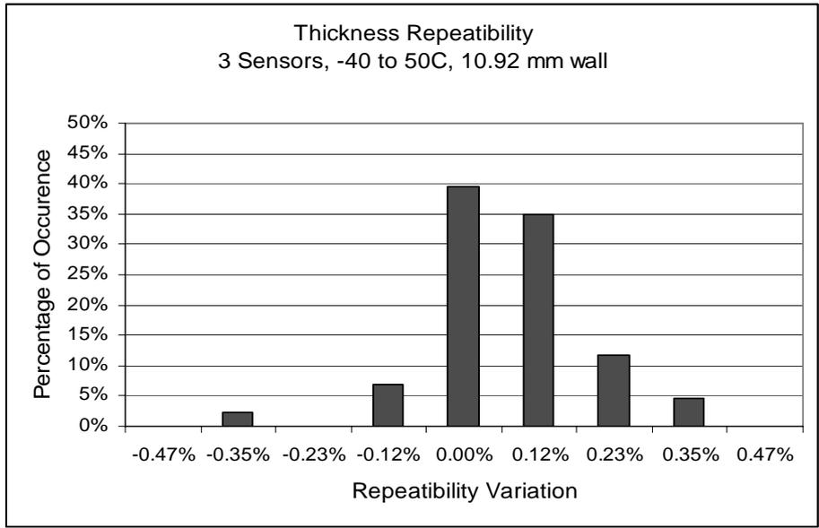
Figure 12: Small spread in data over 90C temperature range and over three sensors is shown
