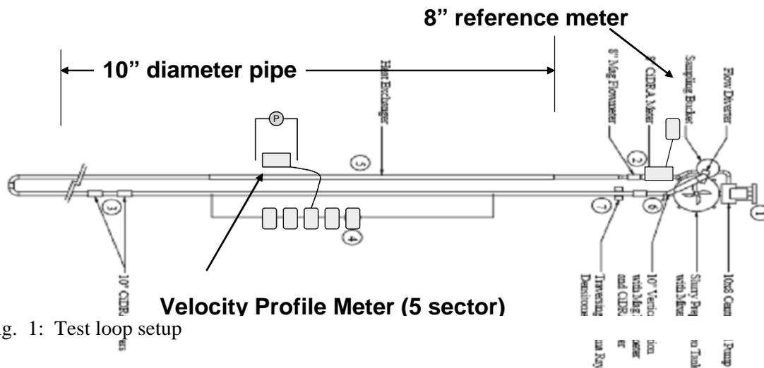
Fig. 1: Test loop setup
