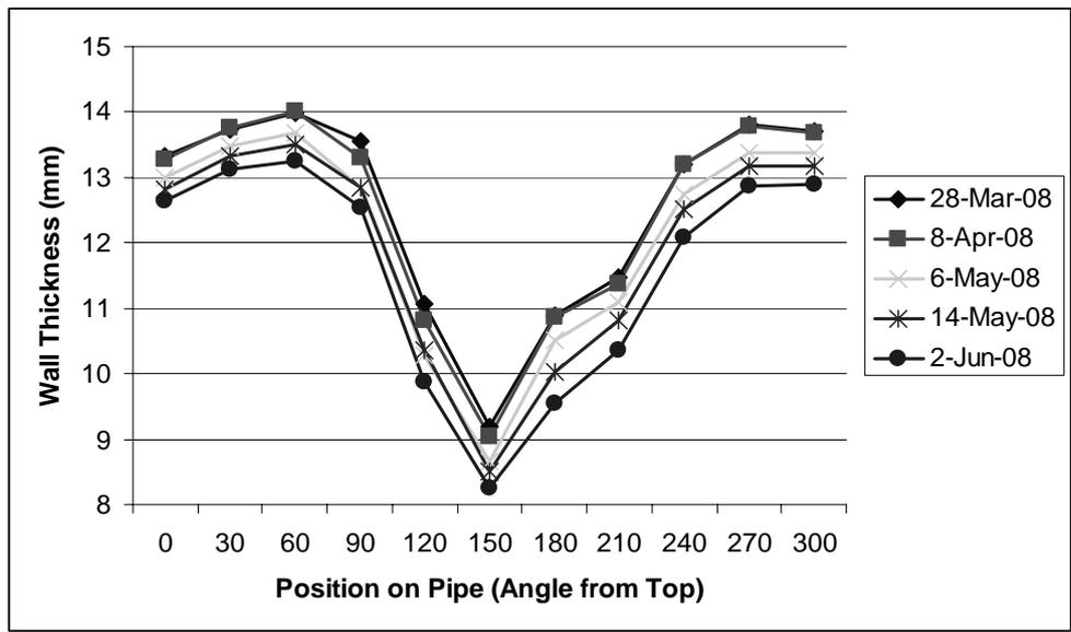
Figure 13: Measurement of pipe wall thickness as a function of angular position and time is shown
