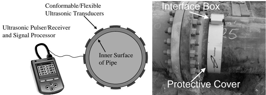
Figure 10: Conceptual layout of HALO™ system and picture of system in operation at a customer site
