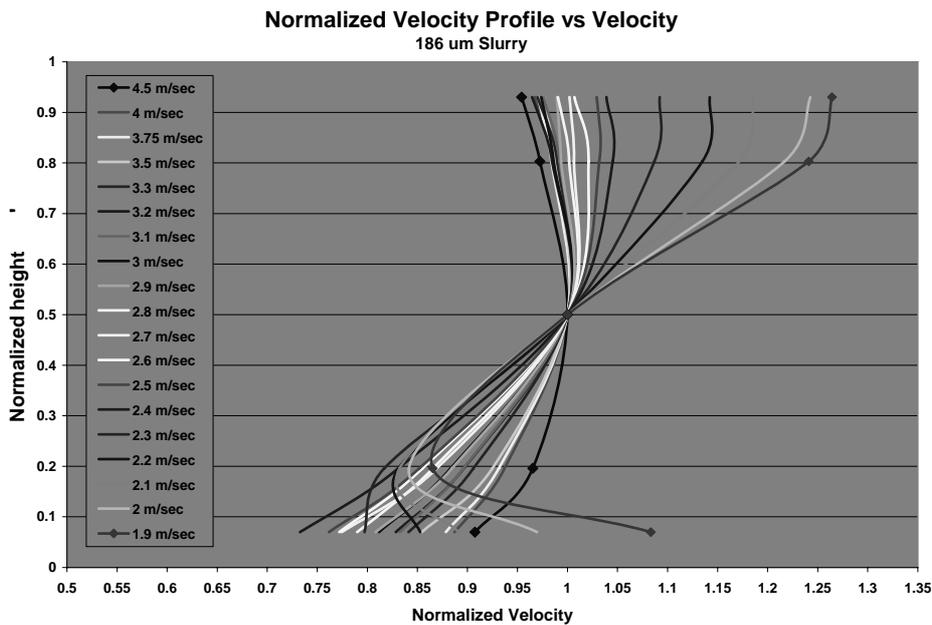
Fig. 9: Velocity profiles (normalized to pipe center velocity) vs reference velocity
