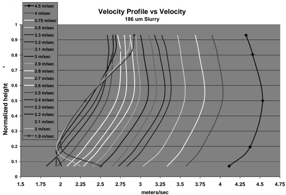
Fig. 8: Velocity profiles vs reference velocity
