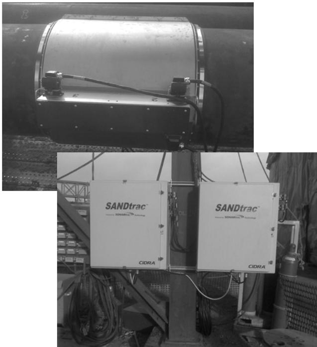
**Figure 12** Operation of velocity profile monitoring system at customer site.
