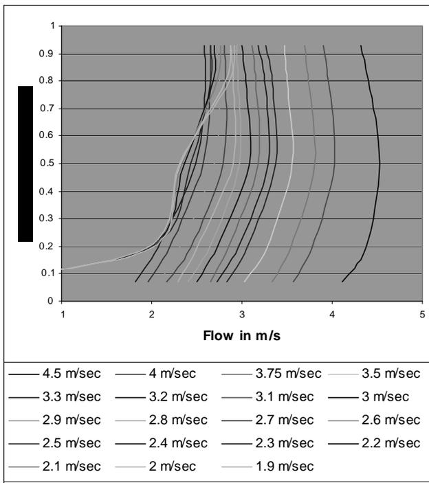
**Figure 10:** Velocity profiles vs. reference velocity
