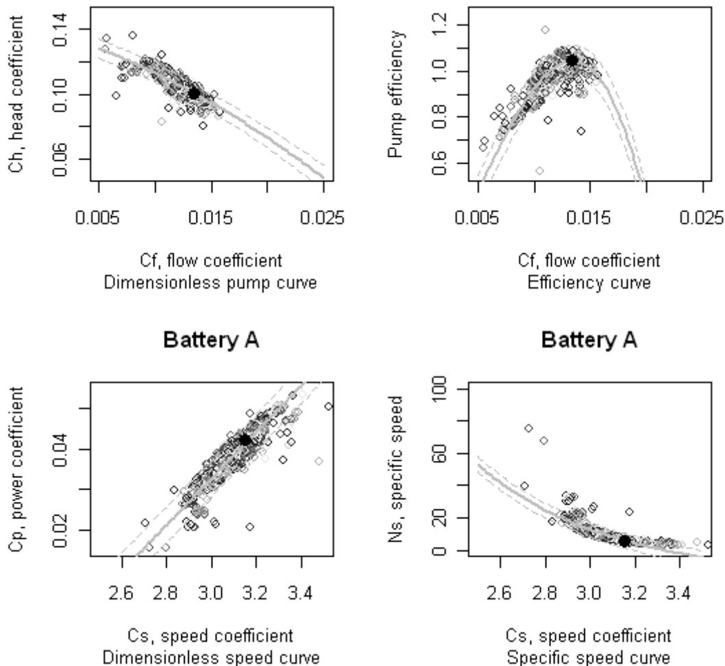
**Figure 3. Four plot of hydraulic dimensionless numbers.**
