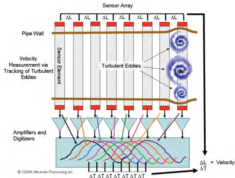
**Figure 3. Illustration of strain induced in pipe walls by passing turbulent eddies, resulting in similar signals detected by sensor elements with time or phase differences, leading to velocity measurement**
