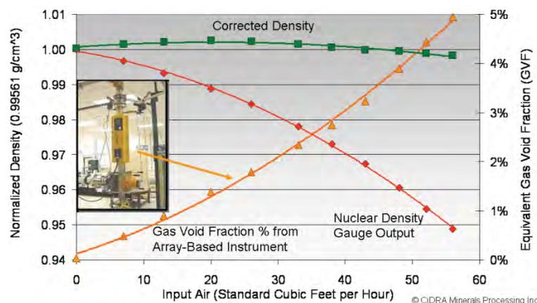
**Figure 12. Nuclear density gauge correction using array-based meter**
