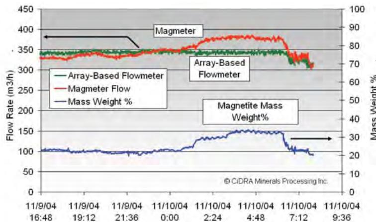
**Figure 6. Electromagnetic flowmeter erroneously respond to magnetite whereas array flowmeter accurately reports flow**
