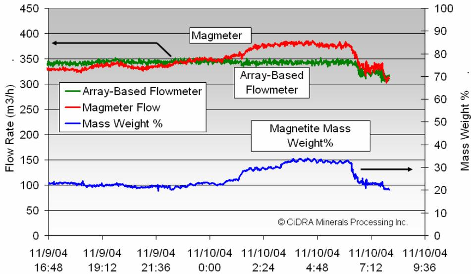
Figure 6 - Electromagnetic flowmeter erroneously respond to magnetite while array flowmeter accurately reports flow
