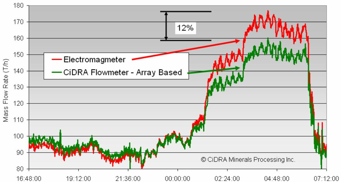
Figure 7 - Impact of ferromagnetic slurry on mass flow rate, showing over-reporting by electromagnetic based flowmeter versus array based flowmeter
