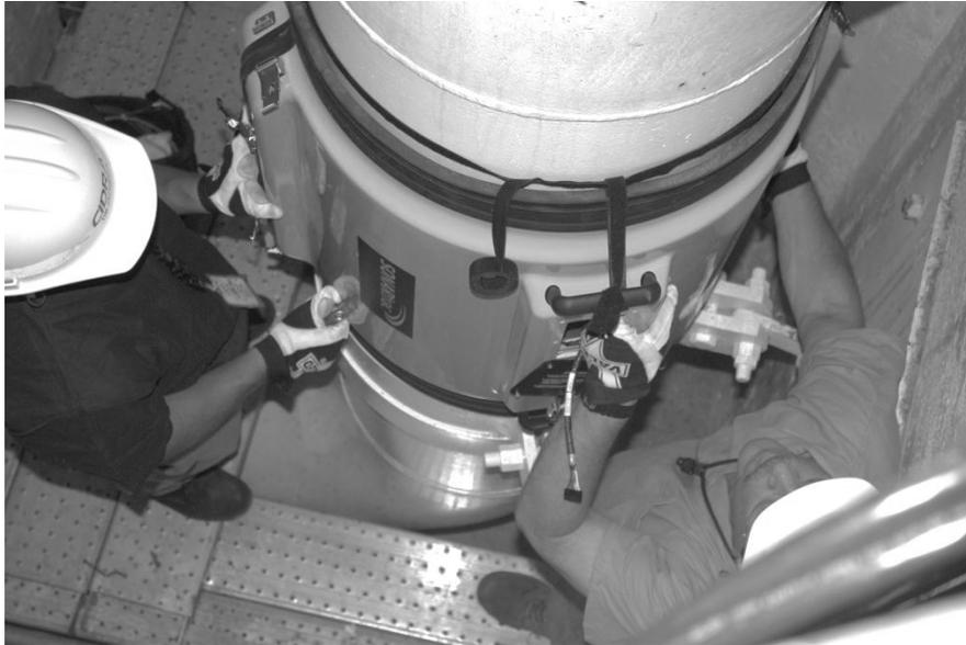
**Figure 11 Sensor Head Cover Installation**
