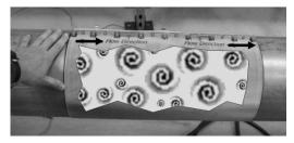
Figure 1: Cutaway of Pipe Under Sonar Array Sensor Band to Illustrate Turbulent Eddies Page 3 of 15
