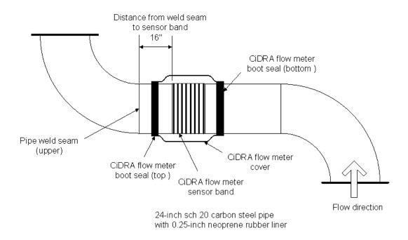
Figure 9 Test Pipe Designed to be Identical to Installation Pipe
