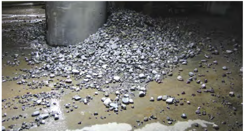
Figure 2—Rock flushed from a rougher row after a significant rock event.
