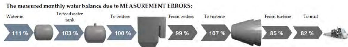
Figure 2 The monthly water balance of a power plant showing the effect of measurement errors.
