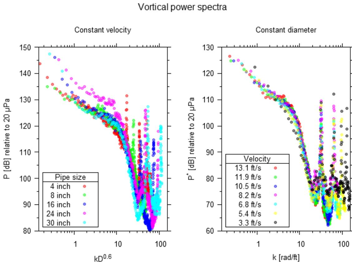
Figure 3 Vortical power spectra
