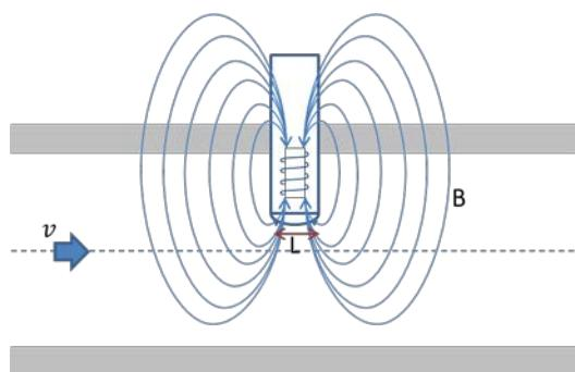
**Figure 6** Insertion mag meter measurement principle
