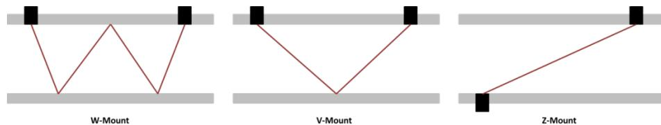
**Figure 2** Transceiver mounting configurations
