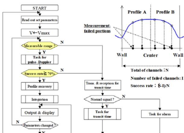
**Figure 4** Hybrid ultrasonic flow meter switchover algorithm
