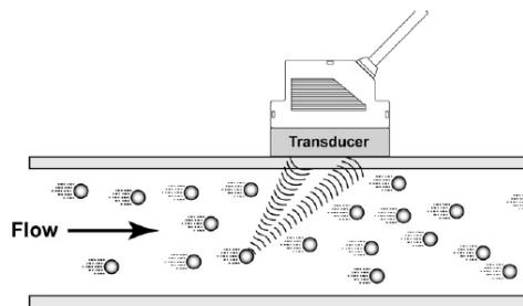
**Figure 3** Ultrasonic wave Doppler frequency shift
