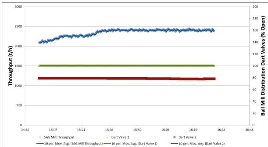
Figure 8 SAG throughput and ball mill distribution dart valve status over same 1.5 hour time period
