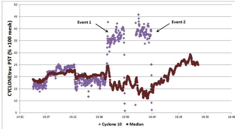
**Figure 6** CYCLONetrac PST measurement (% +100mesh) on cyclone 10 and the average PST measurement for all operational cyclones over a 1.5 hour time period
