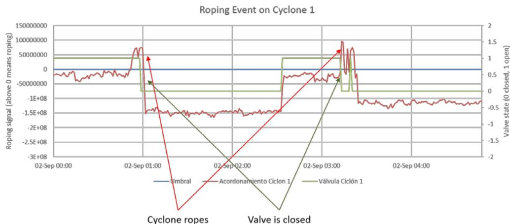
Figure 3 Typical operator response to roping event
