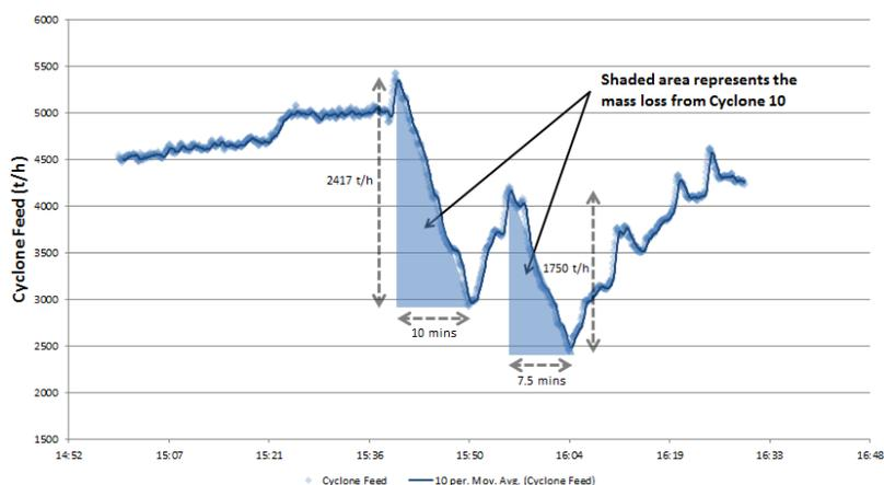
**Figure 9** Feed to cyclones in tons per hour over same 1.5 hour time period
