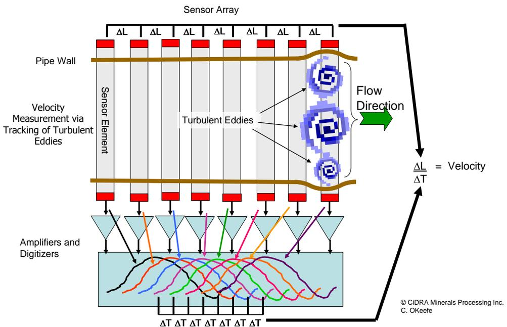
Figure 2 - Illustration of strain induced in pipe walls by passing turbulent eddies, resulting in similar signals detected by sensor elements with time or phase differences, leading to velocity measurement
