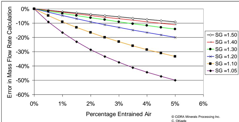
Figure 7 - Error introduced by entrained air in mass flow rate calculations as a function of slurry relative specific gravity (SG)
