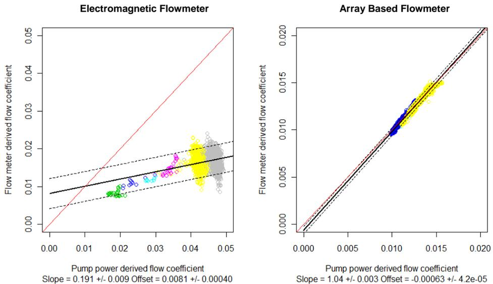
Figure 11 - Flowmeter coefficient versus pump power coefficient for electromagnetic flowmeter and array-based flowmeter
