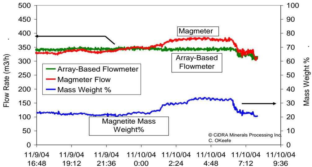
Figure 5 - Electromagnetic flowmeter erroneously respond to magnetite while array flowmeter accurately reports flow
