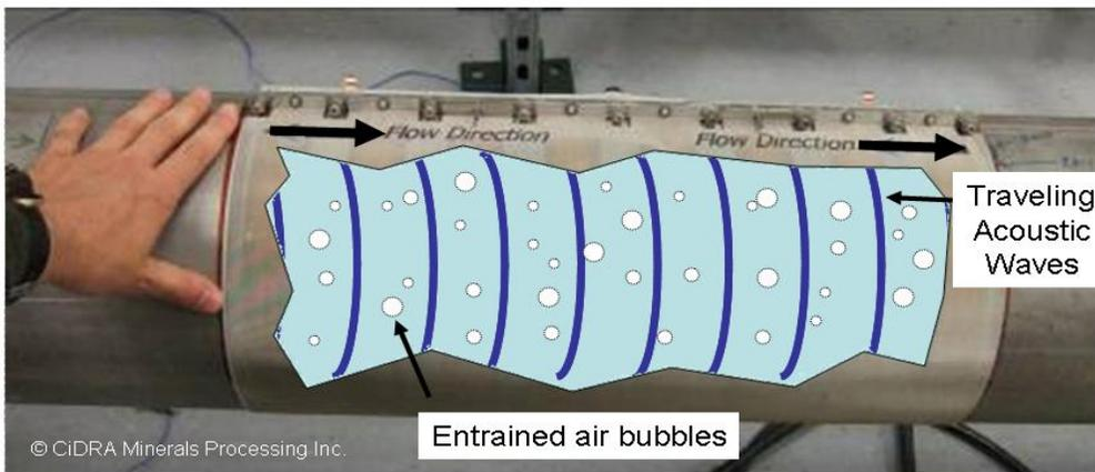
Figure 3 - Illustration of naturally occurring acoustic waves propagating in pipe under the array of sensors
