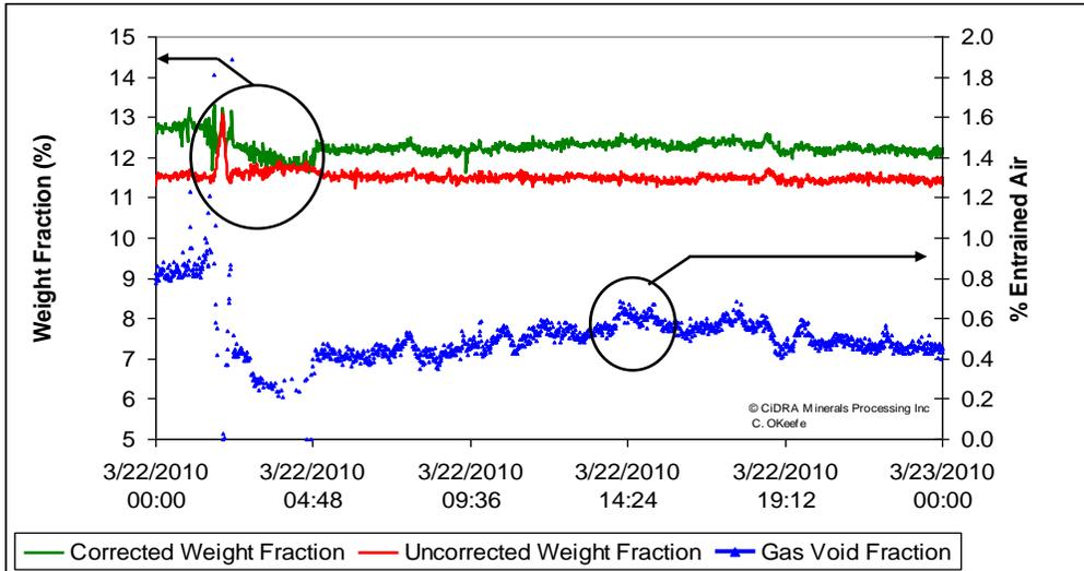
Figure 9 - Solids weight fraction corrected for entrained air content (Gas Void Fraction) and uncorrected weight fraction
