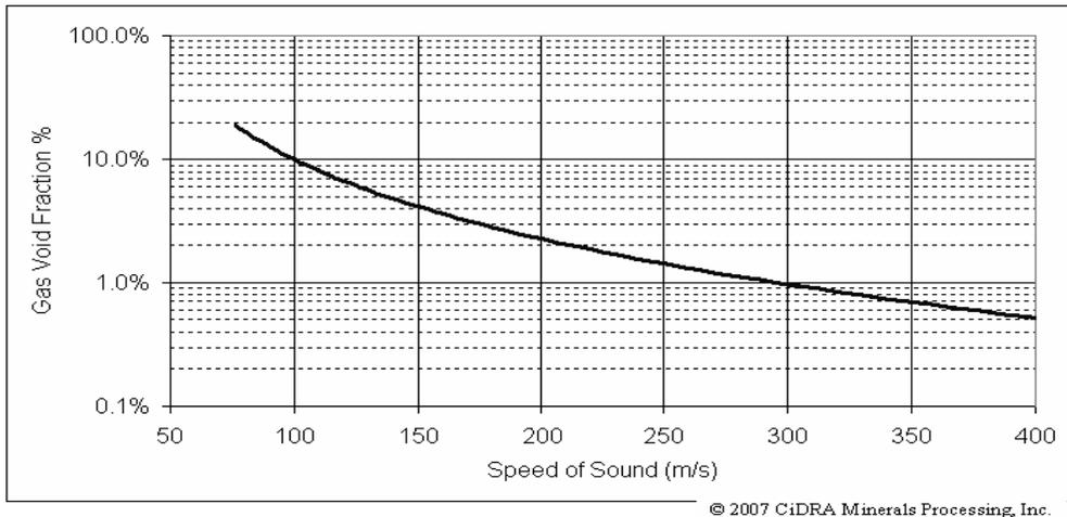
Figure 4 - Example of relationship between gas void fraction (entrained air bubbles) and speed of sound
