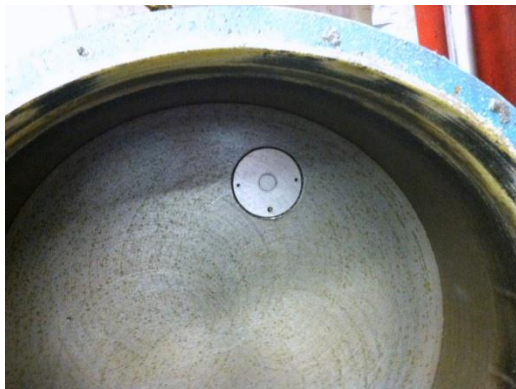
Figure 2: Sensor installed in laboratory pan mixer
