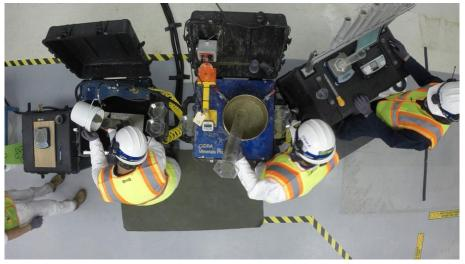
Figure 3 Top view mobile wet sieving and wet slurry analysis stations. The custom shaker shown in middle.
