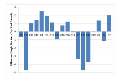
**Figure 4** Difference (Dry stacked sieve laboratory results versus CiDRA's single size wet sieved results). The data nomenclature refers to the cyclone (example: C6 for cyclone six).
