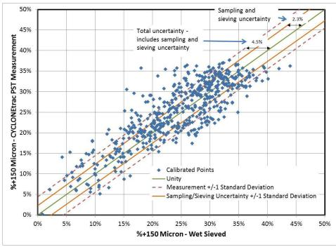
Figure 5 A comparison of the %+150 micron output from the CYCLONEtrac PST probes versus the %150 micron single point wet sieved samples (percentage of solids retained in a 150 micron screen)
