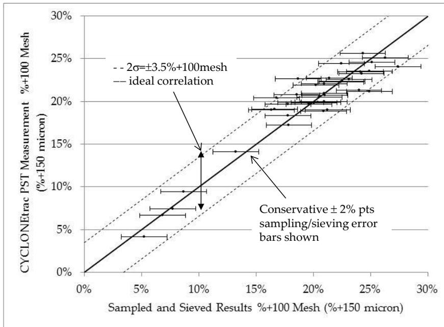
Figure 7 Comparison of CYCLONetrac PST results and sieved samples
