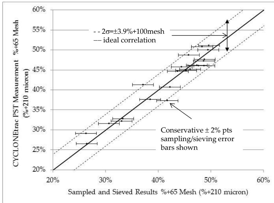
**Figure 6** CYCLONetrac PST 210 micron measurements compared to the sieved samples for a coppery/molybdenum plant.
