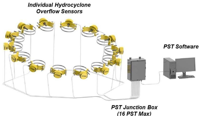
Figure 2. Illustration of particle sizing system.
