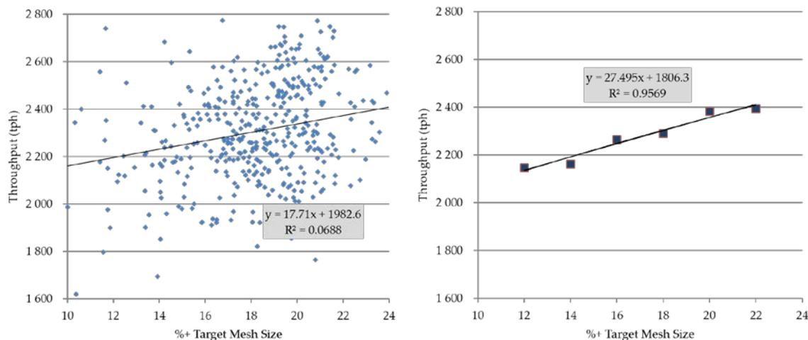
Figure 6 Throughput vs Product Size, with and without data binning
