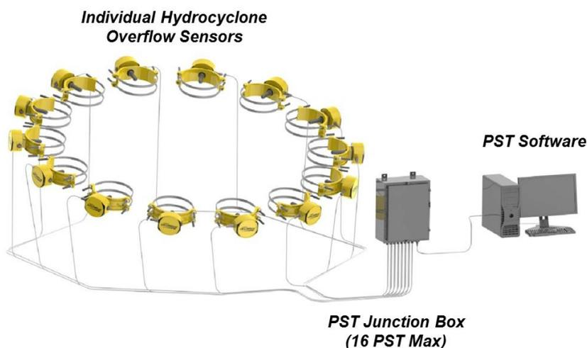
**Figure 2** PST plant scale installation diagram
