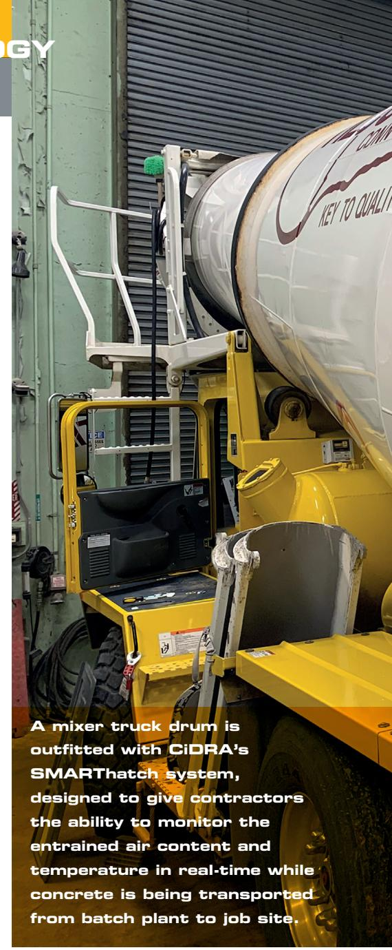
along with GPS data and other metrics, over a 4G LTE cellular interface, to a back office platform, where it can be accessed by remote users. Real time information, including concrete air content percentage, drum speed, concrete temperature and sensor battery level is also sent to a display mounted in the vehicle cab.
