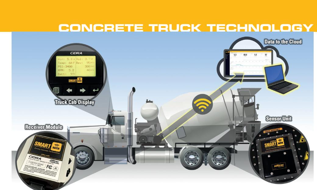
The core of the CiDRA Smarthatch system is the AirTrac system that provides non-contact measurement of entrained air and temperature of the concrete in the mixer truck drum. That information is displayed in the vehicle cab and transmitted to the cloud via HED's CANect Telematics system.
